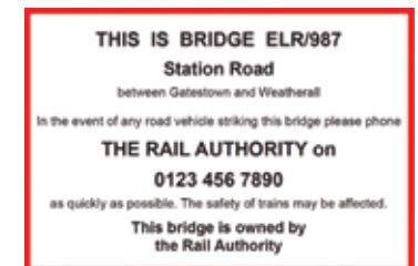
Example identification plate at rail bridge
