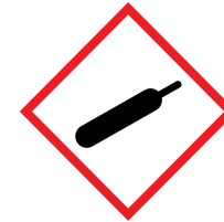
GAS UNDER PRESSURE
