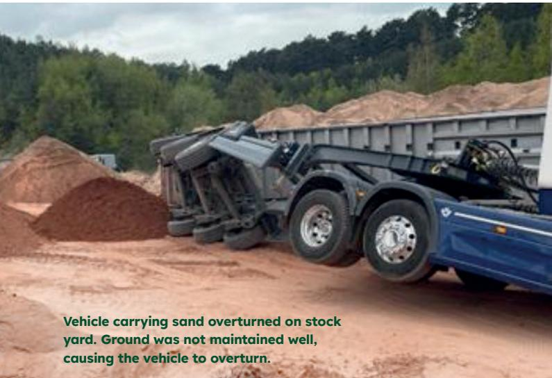
Vehicle carrying sand overturned on stock yard. Ground was not maintained well, causing the vehicle to overturn.
