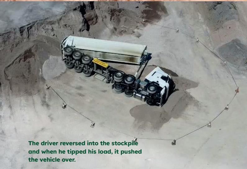
The driver reversed into the stockpile and when he tipped his load, it pushed the vehicle over.
